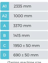
(Taping machine size for boxes W 600 H 600)
