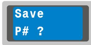
By changing the functions from the "MACHINE FUNCT." list and exiting to the "CHANGE VALUE" page, the system automatically opens this page choose whether to save the changes or not. In this case, by confirming the save, is executed on the active program.
